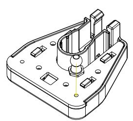
Install the metal pin under the shelf using the pre drillid holes. Attach the soft close support to the arm support (fig.1). Attach the shelf to the track and support arm as shown (fig.2). Install the soft close dampener to the pins (fig.3).
