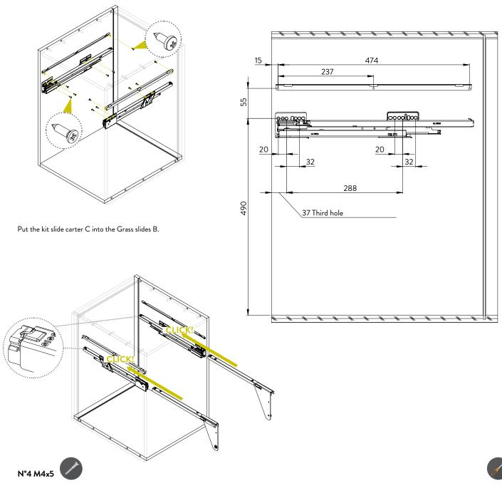
Screw the metal box A into the kit slide carter C by using the specific provided screws.
