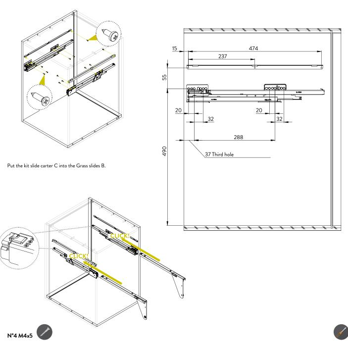
Screw the metal box A into the kit slide carter  $\boldsymbol{C}$  by using the specific provided screws.
