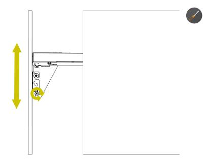
Adjust the door inclination to the front or to the back, than tight the two M6x10 screws.
