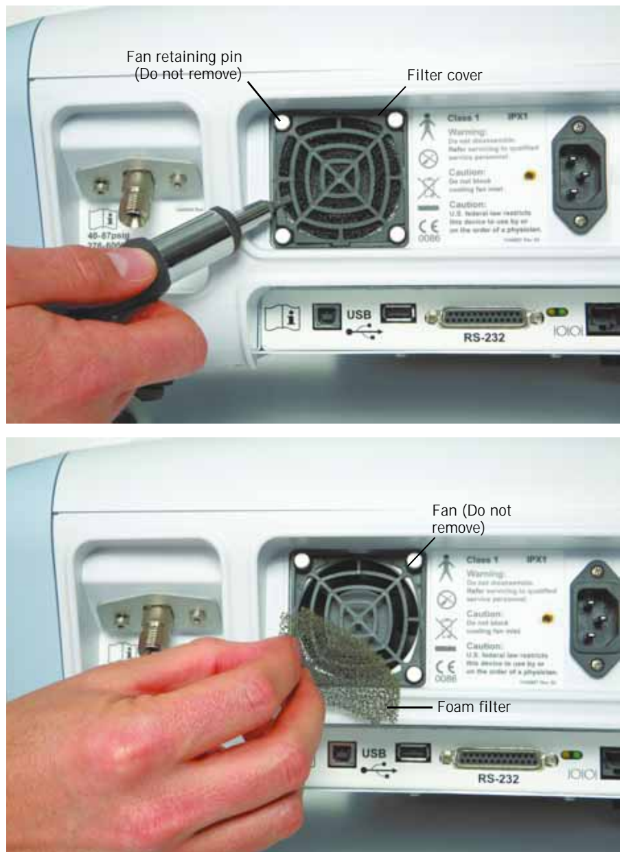
Figure 9-2: Replacing the cooling fan filter
