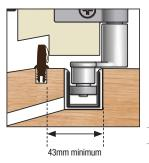
Weathersealing on inward opening configurations can be improved further by using a Threshold Sealing Bar and rebating the bottom edge of the door as illustrated on the left.
