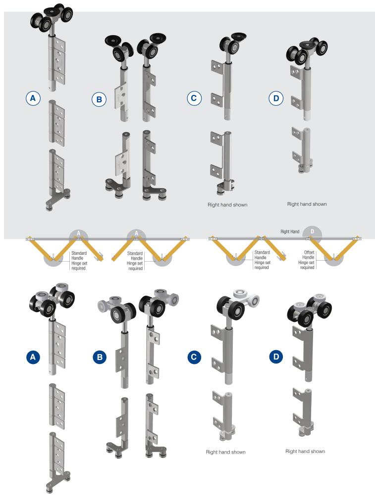
Tommafold carrier sets are at the heart of the system's smooth running and reliability. They come standard with full stainless steel componentry with all wheels having precision ground,
